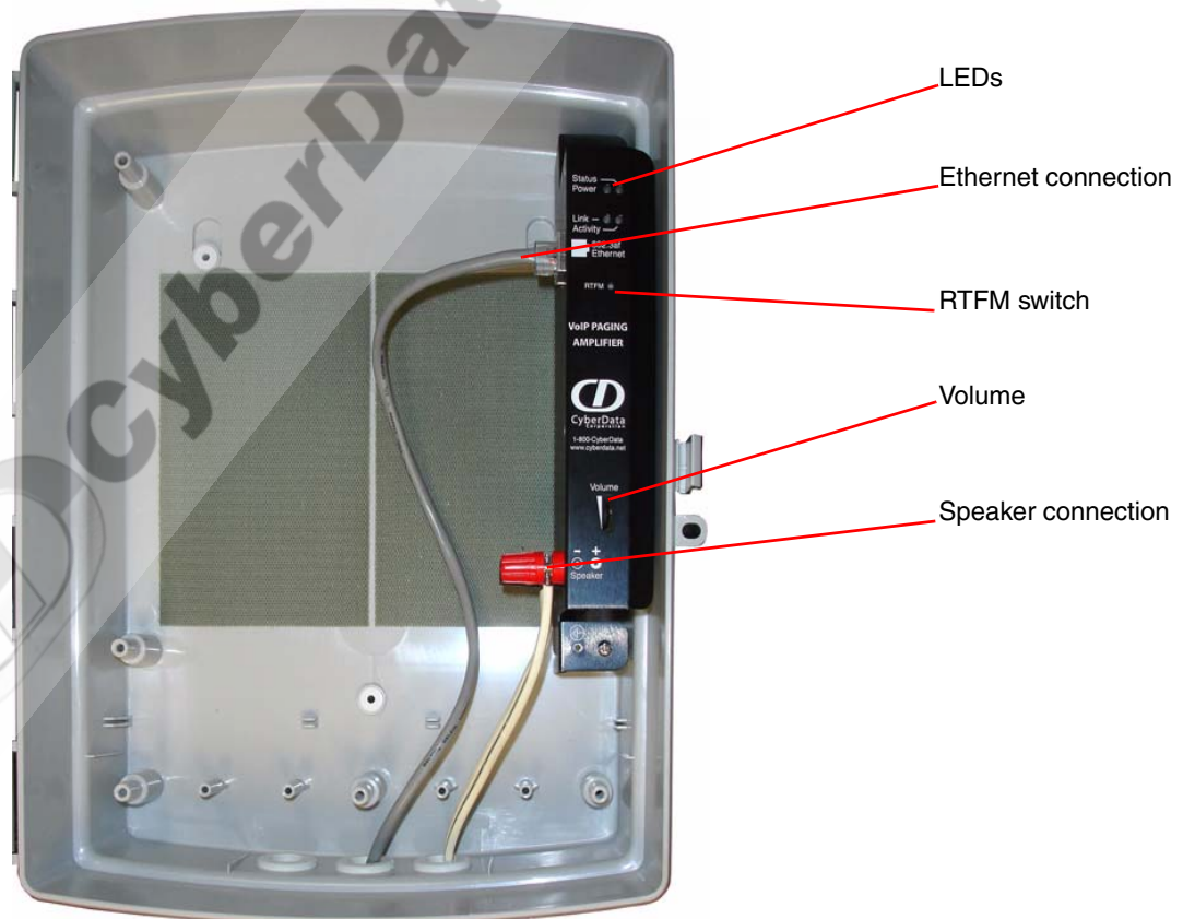
Figure 2-1. Loudspeaker Amplifier Components—PoE
